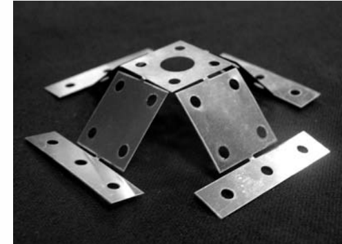
Laser fabricated 4-bar linkage
