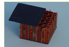
Honeycomb panel is widely used in aircraft structure
