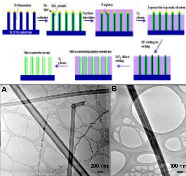
Figure 4 (Top) Flow chart of the fabrication process for making silica nanotube arrays from vertical silicon nanowire templates. (Bottom) Transmission electron micrographs for the as-prepared silica nanotubes.
