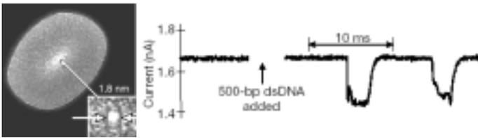
Figure 3 Synthetic nanopore fabricated in  $\text{SiN}_x$  by ion sculpting [16]. Passage of a 500bp double-stranded DNA produces a drop in ionic current in response to a 120 mV bias across a nanopore in the presence of a 1M KCl solution.
