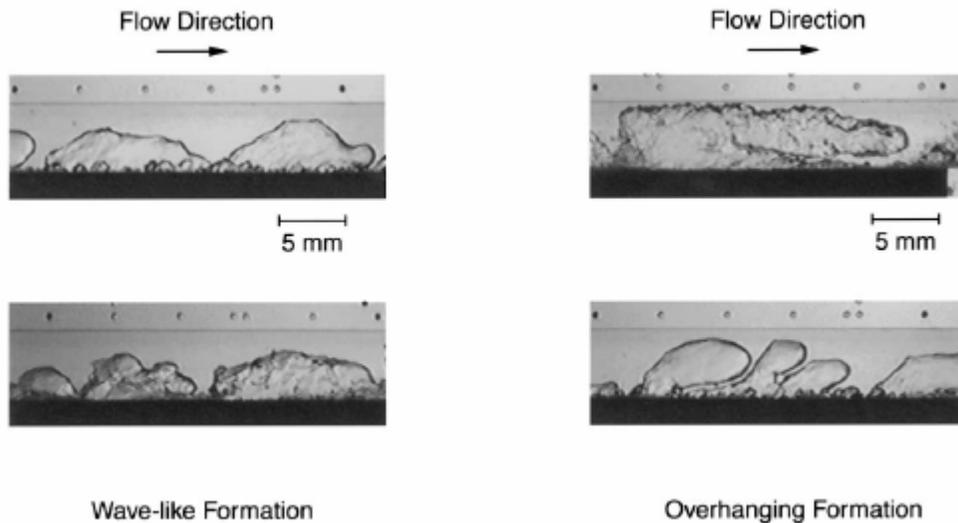
**Figure 5:** Observed vapor structures prior to CHF under subcooled flow boiling conditions.
