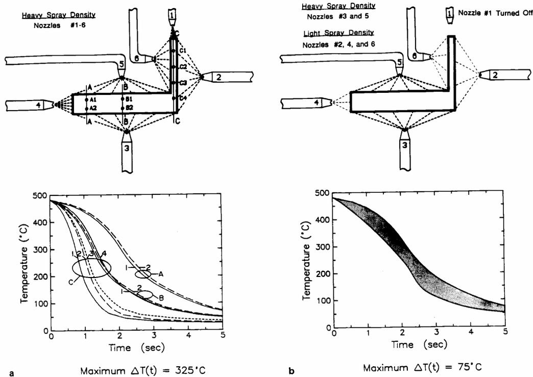
**Figure 3:** Variations with time of temperatures in the solid during quenching under unoptimized and optimized conditions.
