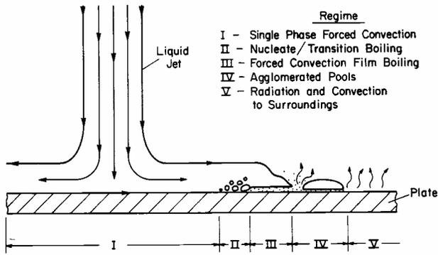
**Figure 1:** Boiling regimes during quenching of steel strip with a planar jet.
