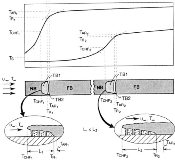
**Figure 2:** Details of quench front region.
