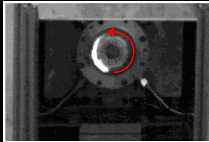
*Rotating detonation engines (RDEs) are the holy grail of propulsion, and Zucrow Labs is helping to bring them to life. Terrence Meyer's lab hosts the THOR (Turbine-integrated High-pressure Optical RDE) test rig, allowing researchers to look inside the combustion chamber, and use laser-based imaging to characterize RDEs' complex dynamics with millions of data points a second.*
