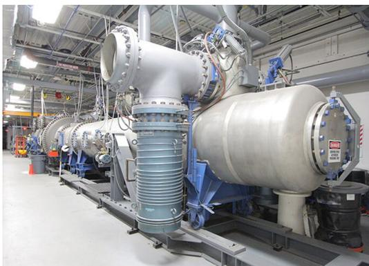
*The HYPULSE hypersonic pulse shock tunnel, donated by Northrop Grumman, is one of several features that makes HARF a unique place to test hypersonic vehicles.*
