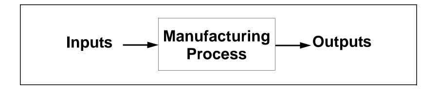
What settings for the process inputs (machine settings, tooling, fixturing, process configuration) provide the desired levels of process outputs (product characteristics: dimensions, finish, microstructure; operation cost, operation time, waste stream flow rates and character) - How??
