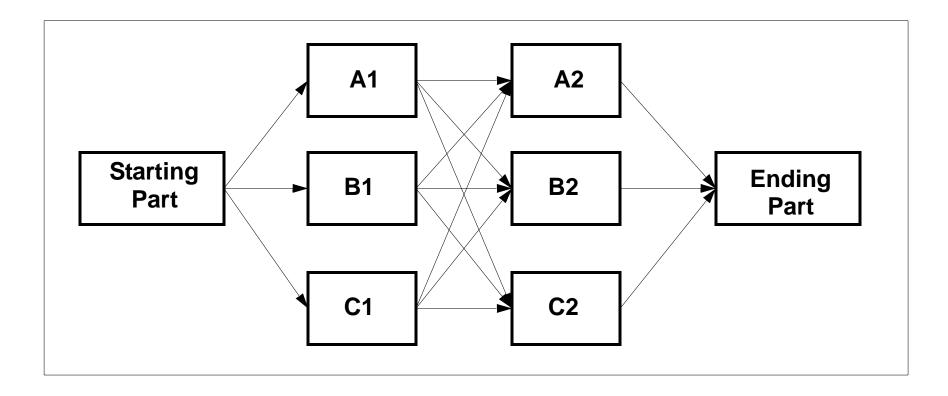
Three alternatives at each step in the sequence -- each sequence consists of two steps.
