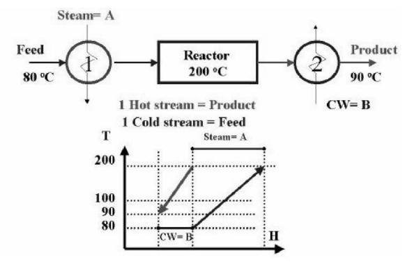
Feed stream to reactor is heated before reactor and product stream is cooled. Heating (done by steam) and cooling (done by cooling water) via heat exchangers.
