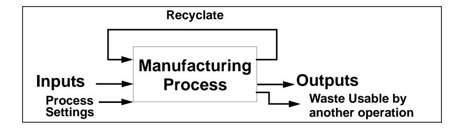
Inputs: Raw material, energy, secondary materials, machinery, air.
