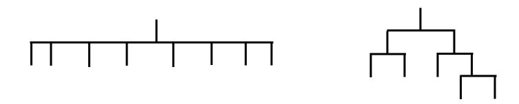
Generally, from an assembly / disassembly standpoint, we are looking for taller hierarchies. Taller hierarchies represent more modular structures.
