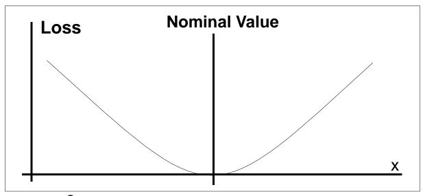
$L = k(x - m)^2$ Loss increases as we move away from the target
