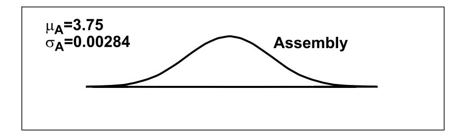
If we again assume that the specs are  $\pm 4\sigma_A$  from the mean/nominal, then the tolerance is  $\pm$  0.01136
