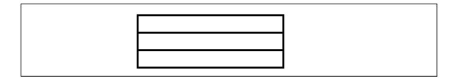
Assembly:  $0.390 \pm 0.050$  inch (0.34 - 0.44) If tolerances are at  $\pm 3\sigma_A$ ,  $\sigma_A = 0.017$
