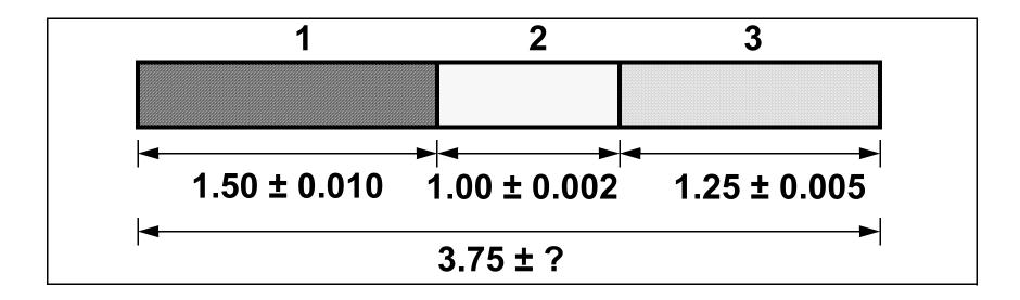
We might naively set the assembly tolerance by simply adding tolerances: ± 0.017
