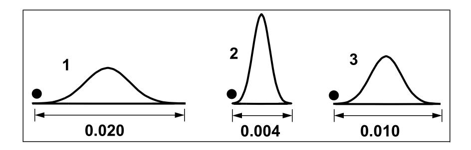
Let's assume specs are  $\pm 4\sigma$  from the mean/nominal Probability of a point at or below  $-4\sigma = 0.00003$  Probability of simultaneously obtaining 3 such points:  $(0.00003)^3 = 2.7$  E-14 (1 in 37 trillion!!)
