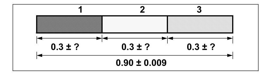
How do we obtain the tolerances on the individual parts? Divide 0.009 by 3 = 0.003 ??
