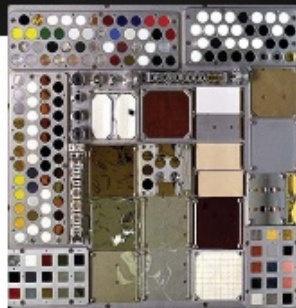
FIGURE 4. The MISSE 7 experiment on the International Space Station was photographed by a space-walking STS-129 astronaut. The experiments expose materials and composite optical and electronic samples (inset) to the external environment; the materials—including solar cells, optics with coatings, sensors, electronics, and structural and protective materials—are evaluated both in situ and after exposure using a variety of instruments such as BLUE-Wave spectrometers. (Courtesy of NASA)
