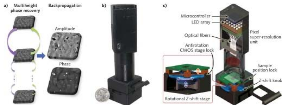
FIGURE 1. a) A multiheight phase-recovery process enables imaging of dense and confluent samples by propagating back and forth between super-resolved holograms acquired at different heights. The resulting complex field is then backpropagated to the object plane, yielding amplitude and phase information of the specimen. b) Weighing only ~122 grams, the lens-free multiheight holographic microscope achieves submicron resolution across a field of view of about 30 mm 2 . c) A schematic of the same device is shown.
