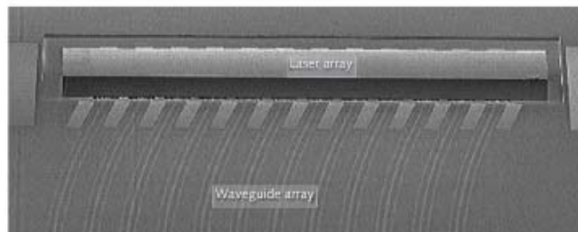
An array of 12 lasers on a single bar are flip-chip-bonded onto a silicon photonics chip and lined up against waveguides.
