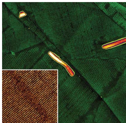
FIGURE 3. A hexacontane sample is prepared and imaged on highly oriented pyrolytic graphite. The “green” image represents the height while the inlay is measuring the elasticity. The stripes are individual monomolecular layers of hexacontane and correspond to the length of the molecule (7.5 nm). The scan size is 5 \mu\text{m}^2 with the inlay being 300 \times 300 \text{ nm} . The z-height scale is 12 nm while the elasticity shows a range of 2.2 GPa.
