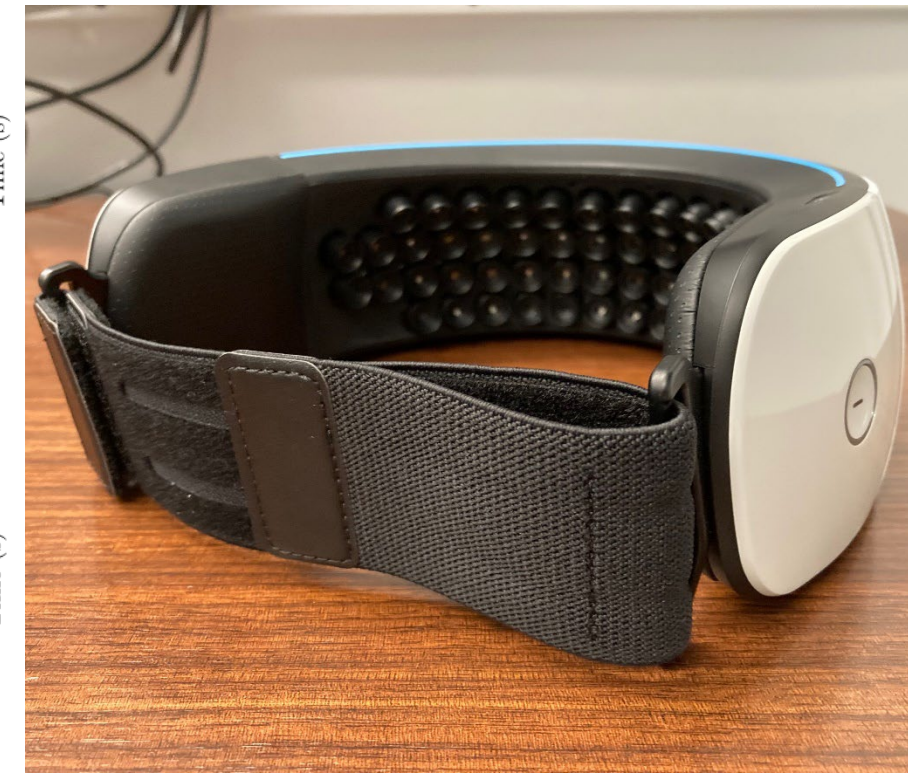
Figure 3: The Obelab NIRSIT fNIRS device is a headset worn on the forehead, covering the prefrontal cortex.
