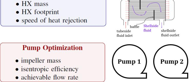
Dynamic HX optimization uses model's eigenvalues to optimize transient performance in addition to design properties
