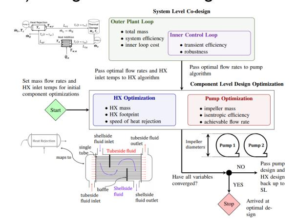
SL co-design algorithm ensures components are connected and operated to optimally to achieve specified performance objectives
