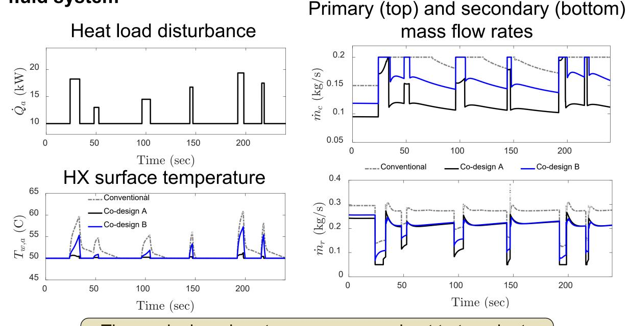
The co-designed systems are more robust to transient disturbances that are common to thermal-fluid systems
