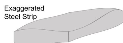
This rotational motion produces periodic disturbances in the thickness profile due to angular variations in the shape and thermodynamic characteristics of the rolls.
