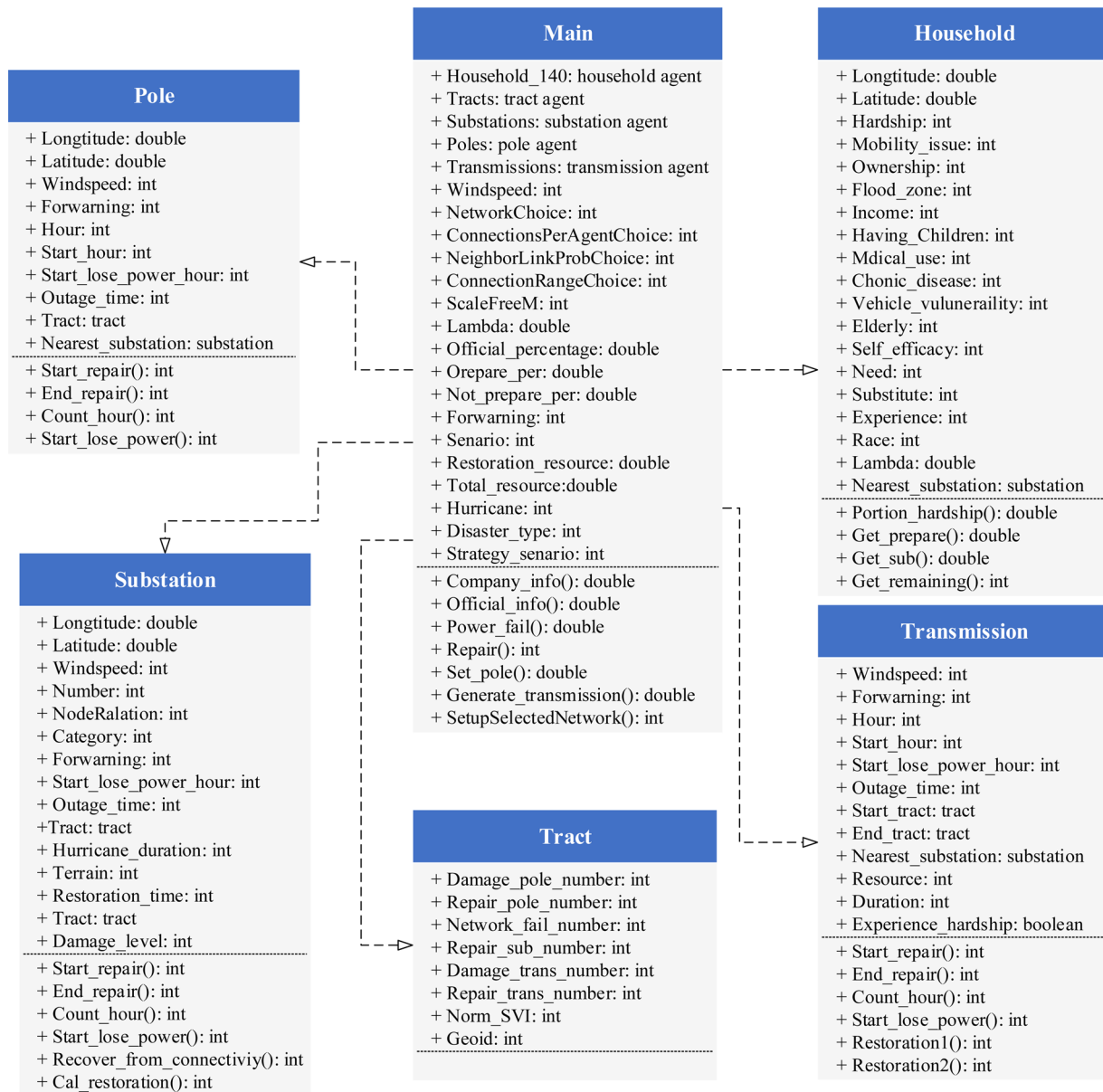
FIGURE 7 Unified Modeling Language class diagram of the multi-agent simulation model
