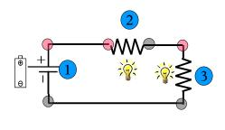
Compare the voltage at position 1 with that at 2 and 3. Compare the currents also. Add the voltages at 2 and 3 and compare with 1 and explain.
