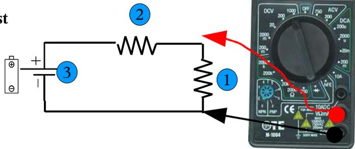
**Step 3: Measure the voltage across the second light bulb in the circuit and record here:**
