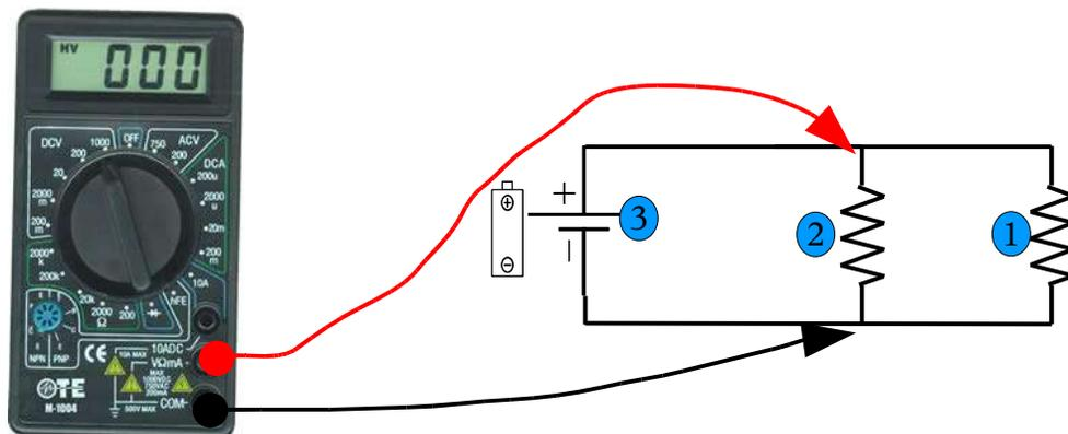
**Step 3: Measure the voltage across the first light bulb in the circuit and record here:**
