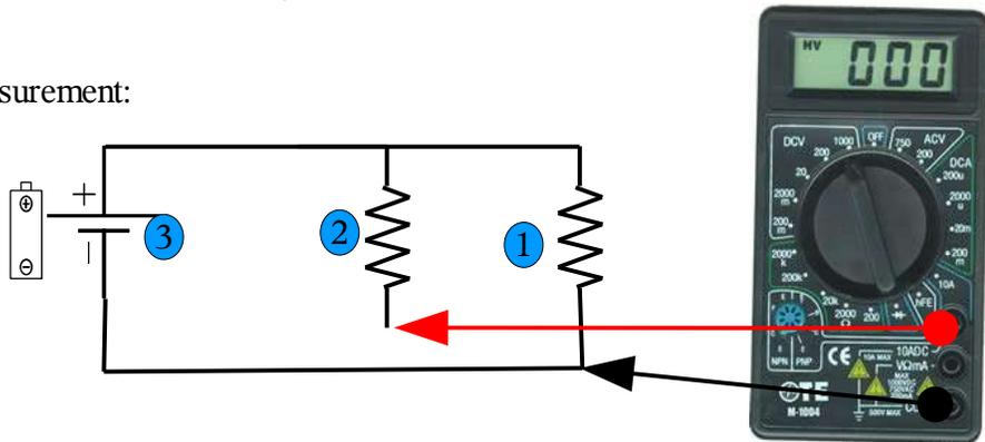
**Step 3: Measure the current between the (-) terminal and BOTH bulbs. This is the current going INTO the circuit.**
