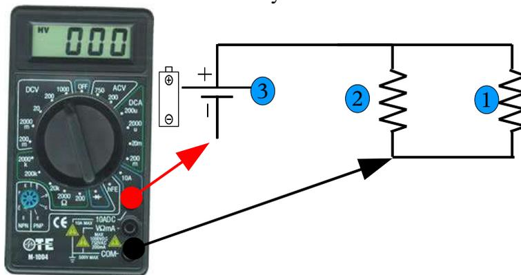
**Step 3: Measure the current between the (+) terminal and BOTH bulbs. This is the current coming OUT of the circuit.**
