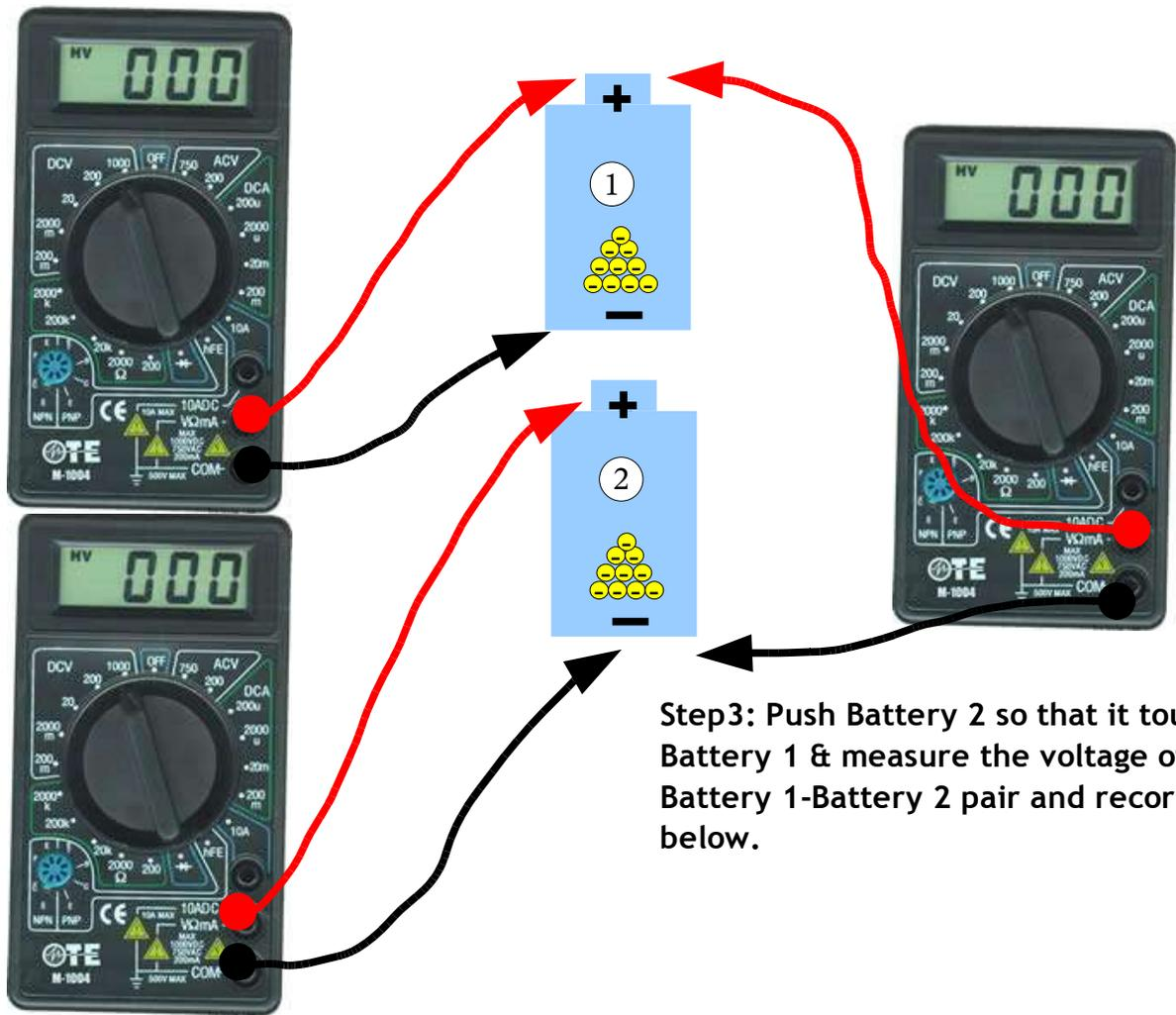
**Step3: Push Battery 2 so that it touches Battery 1 & measure the voltage of Battery 1-Battery 2 pair and record below.**
