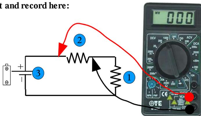
Add the voltages measured at 1 and 2 and compare to the voltage at 3.
