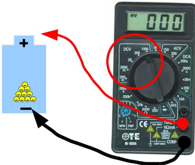
Measure the voltage of Battery 1 and record here:
