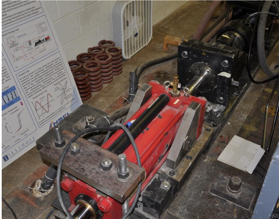
Figure 2.5: UIUC MR damper test setup
