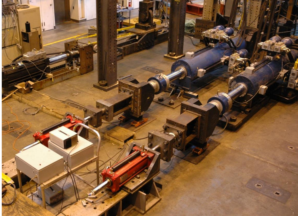
Figure 2.6: Lehigh MR damper test setup
