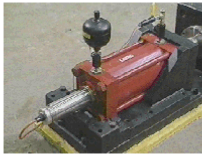
Figure 1.4 180 kN MR damper (Lord Corporation)
