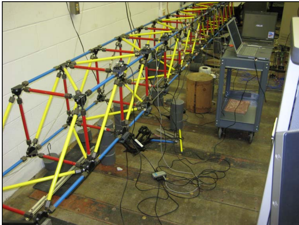
Figure 4.1 3D truss test structure
