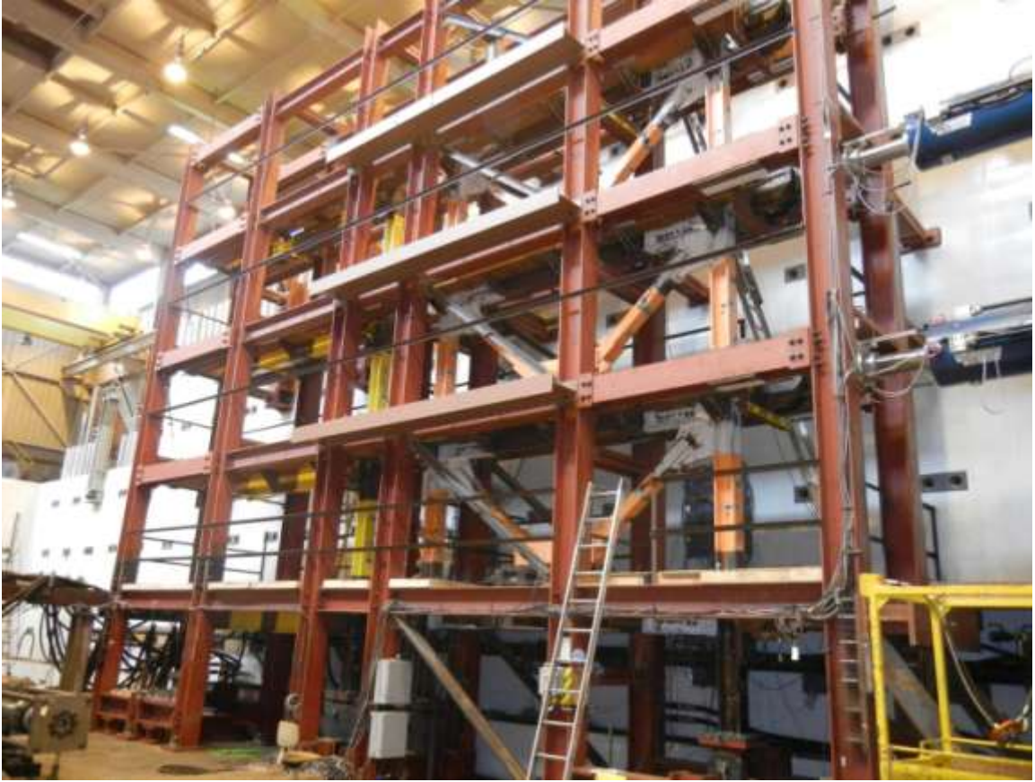
Figure 4.8: RTHS Large-scale Frame Testing Setup at Lehigh University
