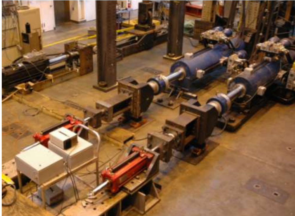
Figure 2.6: Lehigh MR damper test setup
