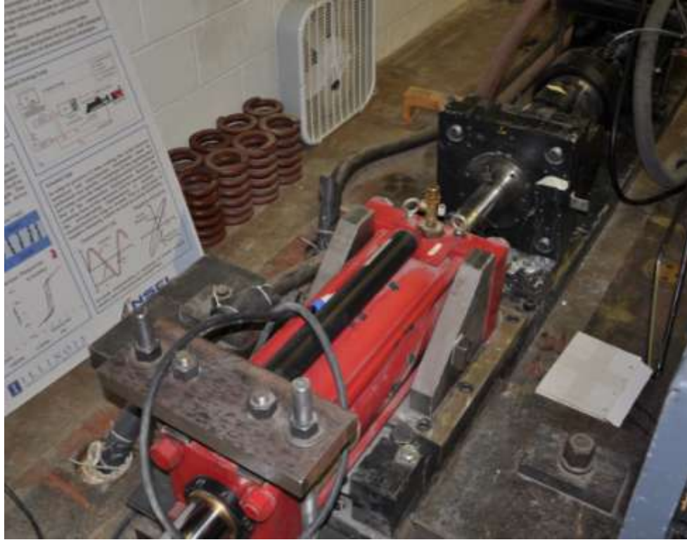
Figure 2.5: UIUC MR damper test setup
