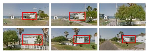
Fig. 3.12.: Reason to observe the house from multiple viewpoints: Optimal rectilinear images with the bounding boxes of the detected house from multiple views. Since the views of the house are partially or entirely obstructed by the foreground objects (here, trees), many images from different viewpoints should be considered to observe the entire front and side views of the house.
