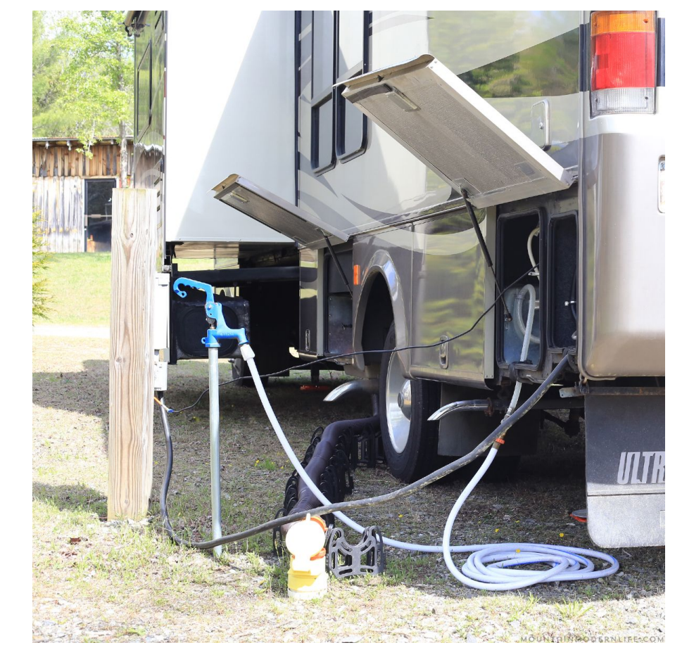
RV Hookup with Water and Electricity
