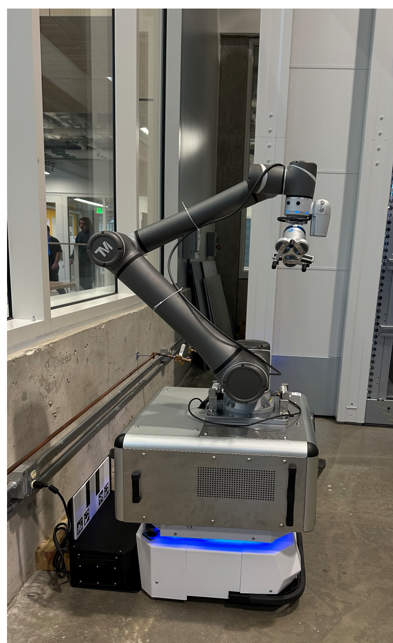
Rosie – robotic arm on moving platform
