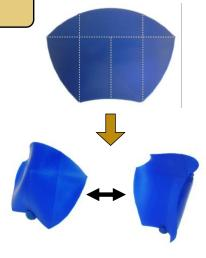
Switchable bistability combines high load carrying capability with low snapping force.
