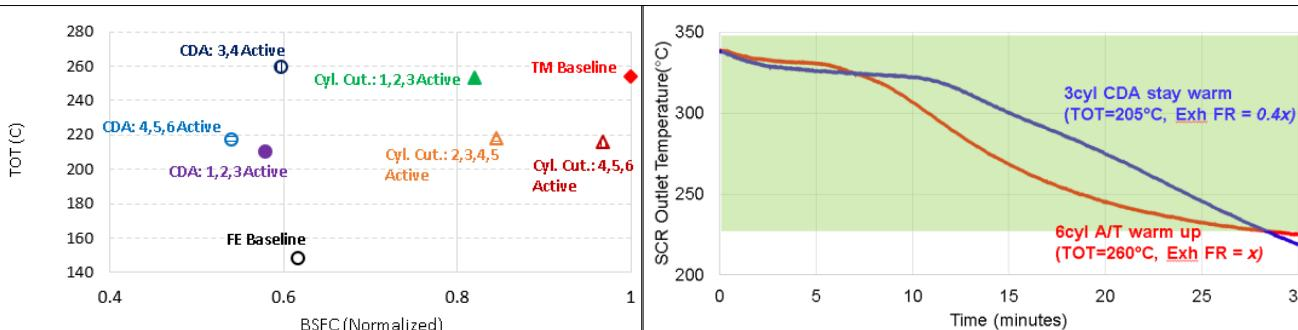
↑ CDA and CCO can provide steady-state idle temperatures similar to the baseline with significant fuel savings
