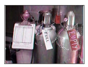
flame shall never be used to detect leaks of flammable gases. Hydrogen flame is invisible, so feel for heat. All cylinders containing flammable gases should be stored in a well-ventilated area.
