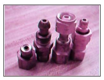
avoided. The threads on cylinder valves, regulators and other fittings should be examined to ensure they correspond and are undamaged.
