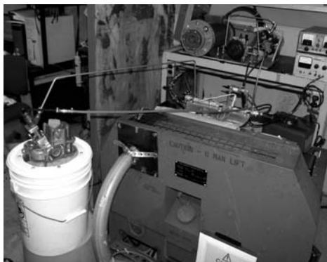
The control development setup, showing the electronic injector sitting over a bucket to catch fuel while the engine is being run with the mechanical injector.
