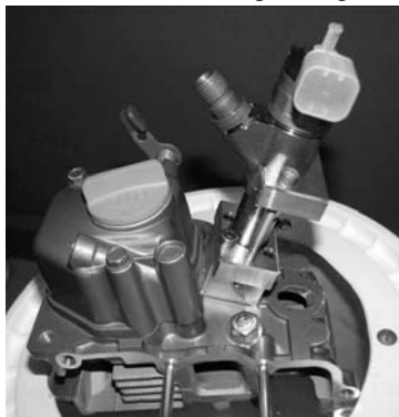
The Bosch electronic fuel injector mounted on the cylinder head.
