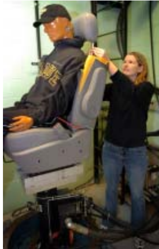
Janette Jaques attaches a sensor to a car seat headrest mounted to a hydraulic shaker. As the seat is shaken, sensors record the vibration data used to validate results from a computational model that simulates the vibration.
