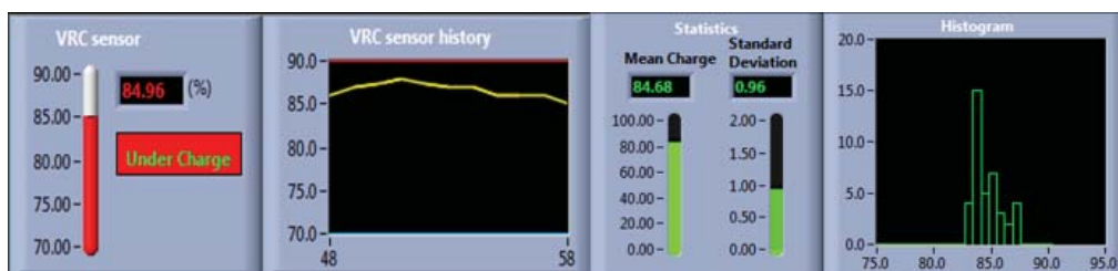
The user interface of the virtual refrigerant charge sensor
