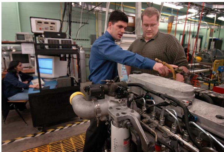
Greg Shaver and Dave Snyder discuss implementing a variable valve actuation system on a Cummins diesel engine.
