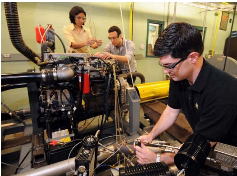
Researchers at Purdue’s Ray W. Herrick Laboratories are developing fuel-flexible combustion control strategies that enable highly efficient, ultra-low emission combustion of both conventional and domestically available alternative diesel fuels, including biodiesel and coal-derived liquid fuels. Gregory Shaver, at right, an assistant professor of mechanical engineering, works with graduate students Gayatri Adi, left, and Mike Bunce to prepare for biodiesel testing with a 2007 Cummins turbo-diesel engine. Graduate student Karla Stricker, in window at right, monitors data acquisition. (Purdue News Service photo/David Umberger)
