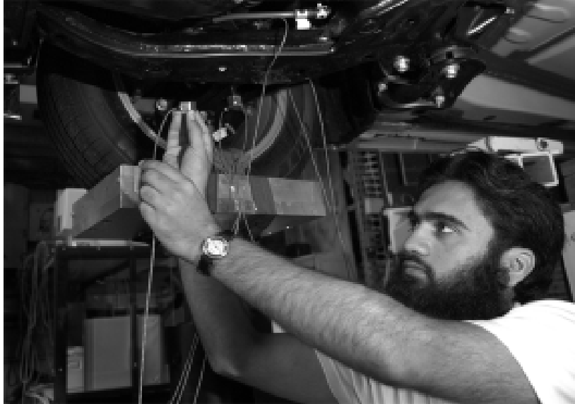
Muhammad Haroon installs sensors in a car suspension system to test out his fault detection monitoring system.
