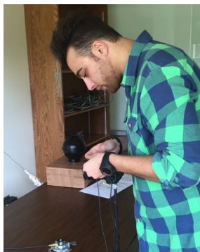
Amir Sadeghi (left) setting up HDR cameras and photometer sensors to measure luminance and illuminance values.
