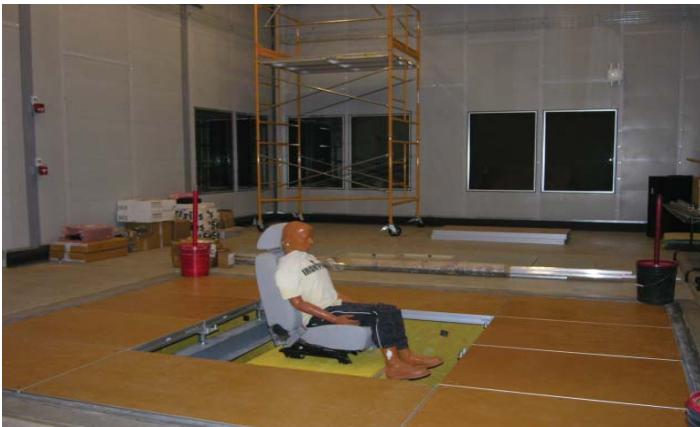
Perception-based Engineering Laboratory showing the 6 degree-of-freedom TEAM shaker
