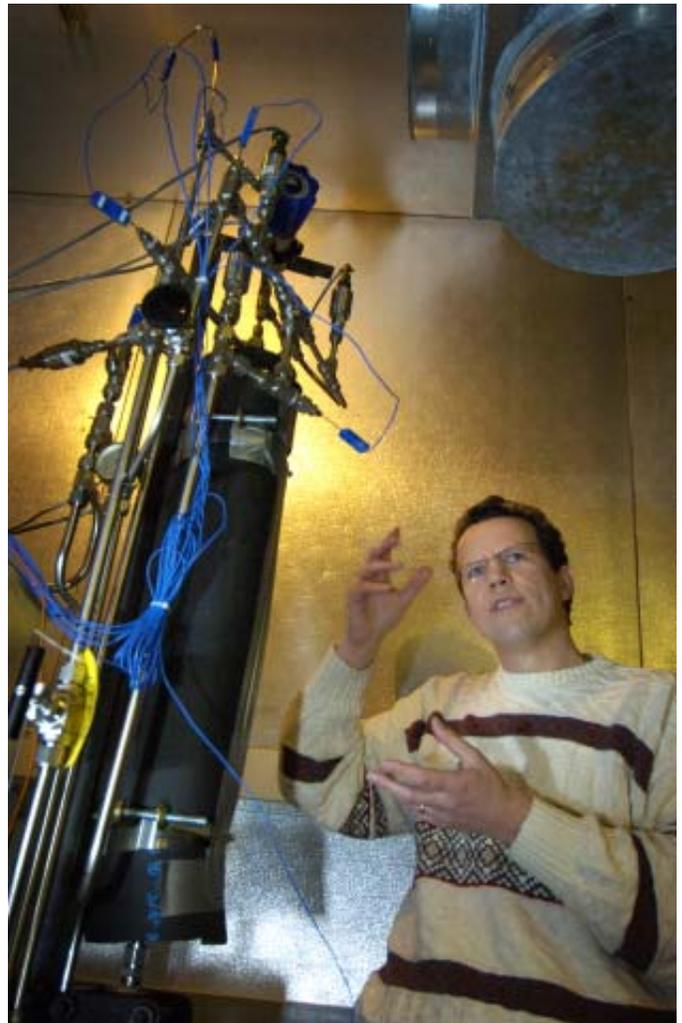
*Eckhard Groll demonstrates a prototype portable air conditioning unit that uses carbon dioxide as a refrigerant instead of conventional chemicals. The prototype has been developed as part of research funded by the U.S. Army. Carbon dioxide is a green alternative to conventional refrigerants, which cause about 1,400 times more global warming than the same quantity of carbon dioxide. (Purdue News Service photo/David Umberger)*
