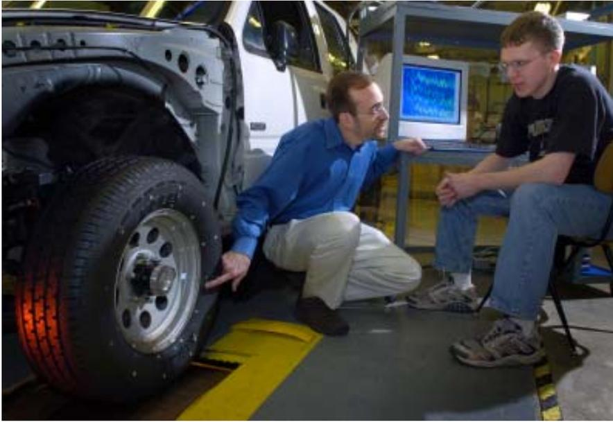
*Douglas E. Adams, left, and doctoral student Timothy J. Johnson use their diagnostic system to detect tire damage as sensor data are displayed in a “wavelet map” on a computer monitor, enabling the engineers to not only detect damage but also possibly pinpoint its location on the tire. The tire-testing research uses sensors and mathematical models to detect defects in newly manufactured tires. (Purdue News Service photo/David Umberger)*
