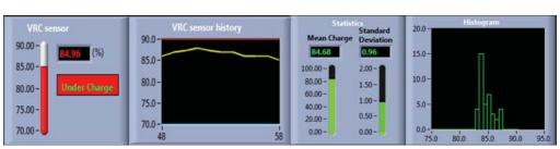
The user interface of the virtual refrigerant charge sensor
