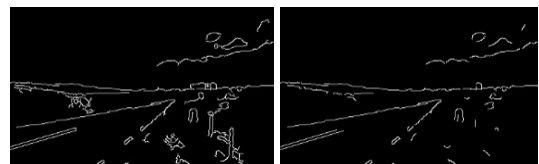
(a) Results of Canny edge detection with using 10 (left) and 100 (right) as the first threshold for the hysteresis procedure
