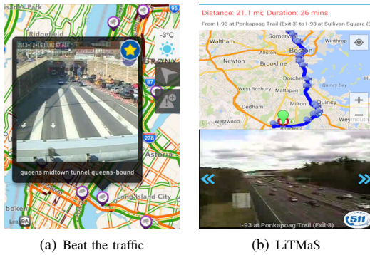
Fig. 1. Existing systems require a user to manually select a camera and show one snapshot at a time; In contrast, LiTMaS provides the user with a video or slideshow of images found from the cameras available along the desired route.
