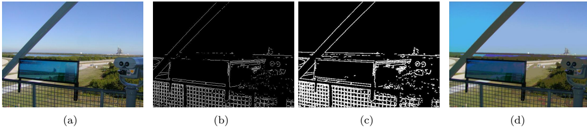
Figure 4: (a) Original image (19.4 KB), (b) Sobel edge image, (c) Edge image determined by our method, (d) New image (15.3 KB). The reduction in size is 21.1%.
