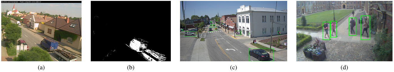
Fig. 6: Sample results of the experiment shown in Table II: (a, b) Motion estimation for a camera in Czech Republic. (a) A sample input image. (b) The corresponding foreground mask. The amount of motion in this image is 5%. (c) Moving objects detection for a camera in the USA. The moving objects are enclosed by green boxes. The image shows eight moving cars, two groups of moving pedestrians, and two traffic lights considered moving due to changing from yellow to red. (d) Human detection for a camera in England. Humans are enclosed by green boxes. The program successfully detects four humans in the image, and misses one.
