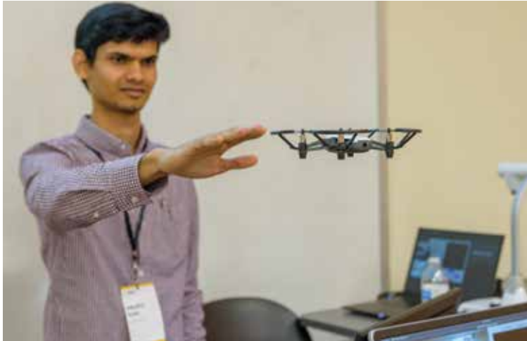
Adarsh Kosta , a PhD student in electrical and computer engineering, controls a drone using hand gestures. Real-time data is captured using a dynamic vision sensor (DVS) and processed using an asynchronous spiking neural network (SNN) processing pipeline that Kosta developed. (Photo credit: Nirmoy Modak)
