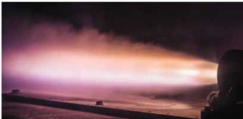
Adranos - one of three companies that has emerged from PERC - performs a static rocket fire test using a high-performance solid propellant for long-range missile and space launch systems.
