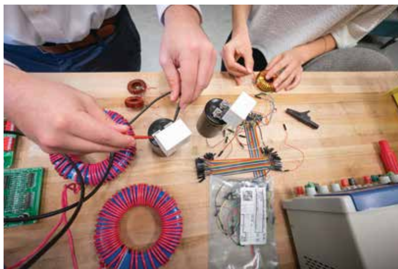
Closeup of power electronic components, used in the compensation circuits of wireless transmitters for inductive electric vehicle charging.
