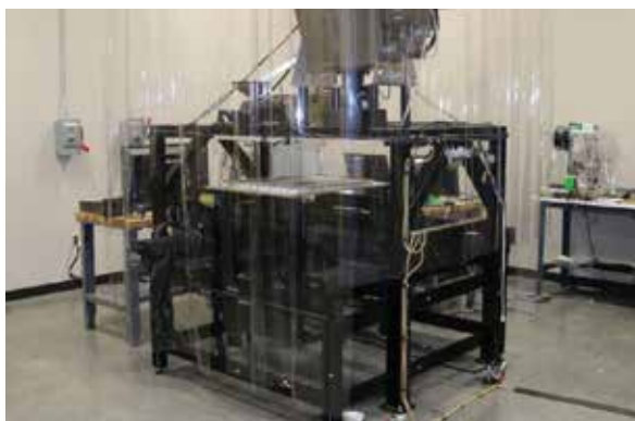
Composites Additive Manufacturing Instrument (CAMRI).
