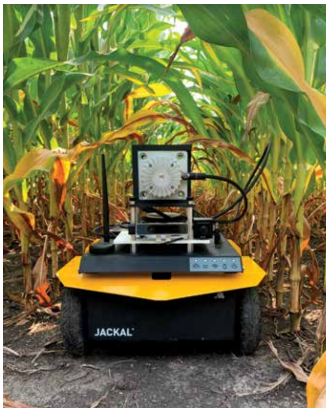
AgBot unmanned ground vehicle (UGV) performs in-row and under-canopy sensing of corn plants at Purdue's Agronomy Center for Research and Education (ACRE) facility. (Image credit: Brian Huang)
