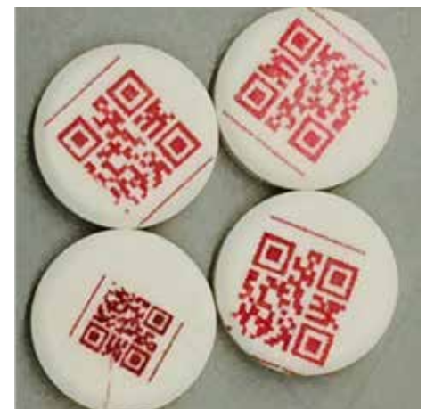
Marking pharmaceutical drugs with QR codes can aid in foiling counterfeiting.
