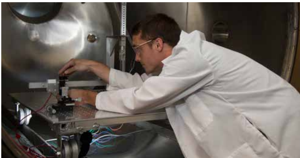
Graduate student Andrew Strongrich prepares a sample to test on a "microNewton thrust stand." Below, Alexeenko holds a component for a satellite microthruster. (Purdue University photo/Mark Simons)
