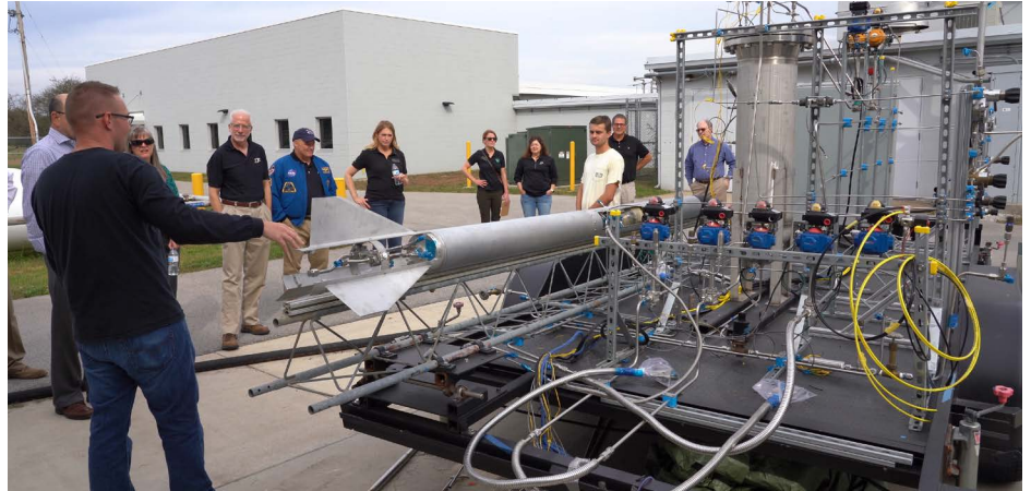
Chris Nilsen of Purdue's SEDS chapter shows off the mobile launch platform for their liquid methane rocket.
