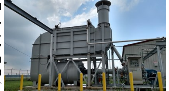
New MZL air heater can deliver 1500 deg. F air at 8 lbm/sec providing capability to simulate compressor exit conditions of most advanced engines
