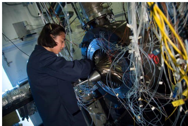
Jeanne Methel, an AAE master's student, calibrates a tip clearance measurement probe for the current centrifugal compressor CSTAR facility. Purdue University photos/Mark Simons
