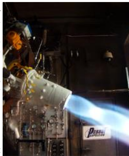
Purdue students have conducted the first 'hot-fire' test of the rocket, which uses liquid oxygen and liquid methane propellants. The students have designed, built and tested a central part of the new engine called the thrust chamber or combustor as part of NASA's Project Morpheus.
