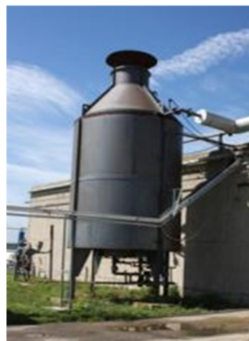
Figure 2: Current MZL Air Heater (r) and Performance at Various Flowrates (l)
