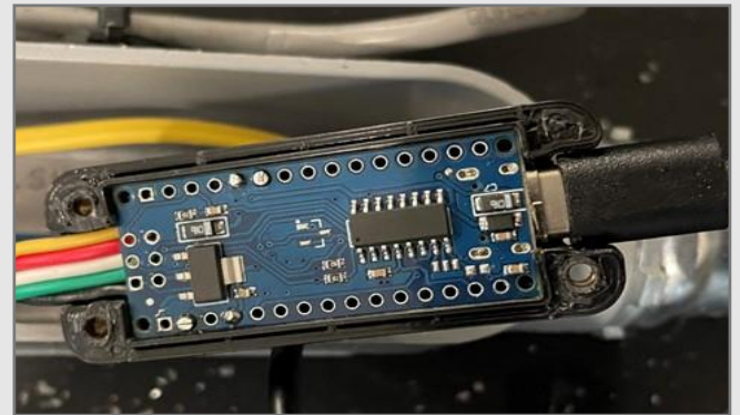
Fig. 2 – Updated Arduino-based Encoder Serial Converter Module
