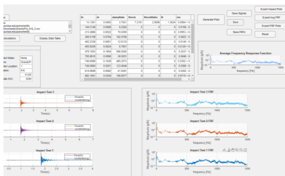
Fig. 3: MATLAB GUI results for Head Gravity Pro at Impact Location 6-8
